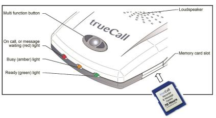
If trueCall detects an error on the memory card you will hear the message "Error on memory card - please remove the card". It may be that the card is faulty, isn't a genuine trueCall card, or just hasn't been inserted fully. Remove the card for 10 seconds then replace it making sure that the card is plugged firmly into the socket.
